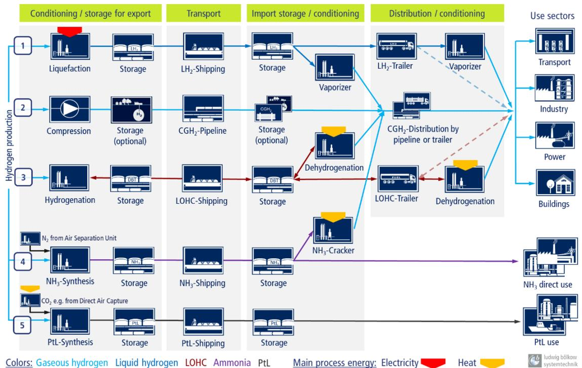
**Figure 23:** Main elements of large-scale hydrogen export/import supply chains (1) LH<sub>2</sub> via ship, (2) CGH<sub>2</sub> via pipeline, (3) LOHC via ship, (4) NH<sub>3</sub> via ship, and the supply of PtL for comparison (5)
